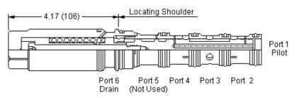
This valve is a 3-way, 3-position proportional directional valve. Port 3 is closed in the center position and port 2 and port 4 are drained to port 1. Pilot pressure at port 1 creates a metering orifice between ports 3 and 4 that is proportional to the pressure at 1. Piloting 6 opens 3 to 2. The force balance of the flow forces, spring and pilot pressure results in a degree of partial self-compensation as the load pressure changes.
