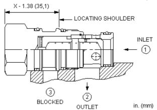
Free-flow, nose-to-side cheater check valves function as a standard 2-port check valve in a 3-port cavity with port 3 of the cartridge blocked off. These valves are useful in circuits where a check valve is required in an existing three port cavity.
