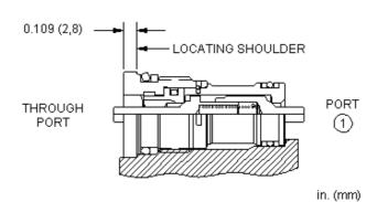
The phaser check is a pair of checks, back-to-back, with both poppets mechanically actuated. The valve is meant to be installed into the piston or rod of a cylinder. When the cylinder reaches the end of its stroke the poppet in the phaser check is shoved off its seat allowing flow through the piston. This allows two cylinders to get back into
