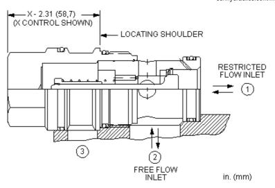
Free-flow, side-to-nose cheater check valves with a bypass orifice function as a 2-port check valve in a 3-port cavity. They allow free flow from port 2 to port 1 with a customer specified orifice that controls flow from port 1 to port 2. Port 3 of the cartridge is blocked off.
