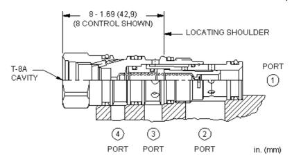
This valve is a, 3-way directional cartridge (1 blocked, 2 to 3 open) that incorporates an integral pilot control cavity. It may be used by itself or to actuate larger pilot-operated directional cartridges or logic elements. The valve shifts when there is flow through the pilot control cartridge installed in the T-8A cavity.
