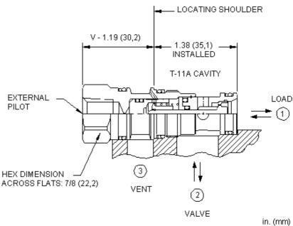
This valve is a pilot to open check valve. It has a non-sealed pilot, a steel seat, and is vented. It allows free flow from the valve (port 2) to the load (port 1) and blocks flow in the opposite direction. Pressure at the external pilot port will open the valve from port 1 to port 2. Pilot pressure needed to open the valve is directly proportional to the load pressure at port 1. The valve is insensitive to pressure at port 2 because the spring chamber references the vent (port 3).
