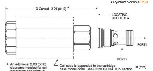
This valve is a pilot-operated, normally open, electro-proportional throttle with reverse free-flow check. Energizing the coil generates a closing force on the pilot stage which pushes the main stage poppet against the seat, proportionally blocking flow from port 2 to 1. In the open condition, flow from 1 to 2 will cause the valve to autoclose and only pilot flow will pass from 1 to 2.
