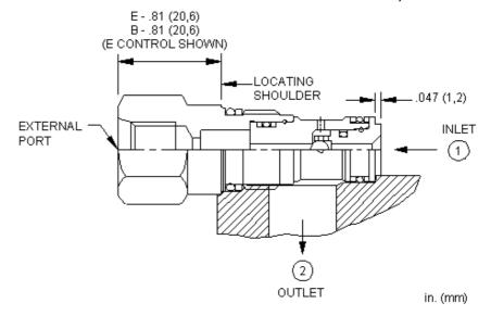
The single ball shuttle connects the higher of two work ports to the signal or common port. It features an external load port located in the hex-end of the cartridge and the signal is sensed at port 2.
