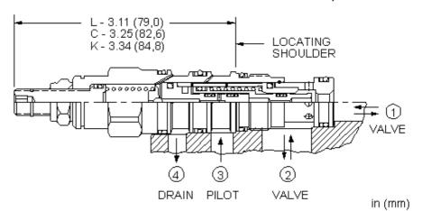
This is a normally open, balanced poppet, switching element. When pilot pressure is applied to port 3, the poppet remains open until the pilot pressure reaches the setting established by the integral pilot relief stage, at which point the poppet shifts to the closed position.
