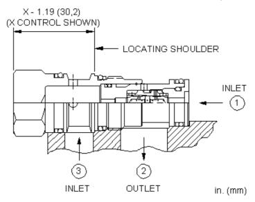
The back-to-back check valve combines two simple check valves into a single cartridge. It connects the work port with the higher pressure to the signal or common port. The signal is sensed at port 2.
