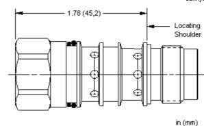
These cavity plugs can be used for both four-port and six-port cavities. In both cases, all ports remain open.
