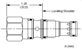
This cavity plug allows ports 2 and 3 to remain open and blocks port 1.
