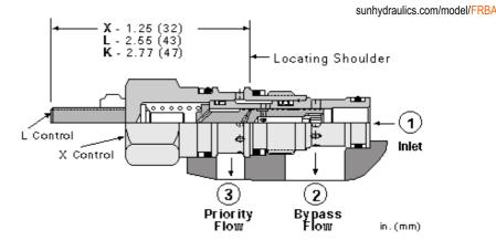
Bypass/restrictive, fixed-orifice, priority flow controls take an input flow at port 1 and use it to satisfy the priority flow at port 3. If the input flow exceeds the priority flow requirement, the excess is bypassed out port 2. The bypass flow may be used in a secondary circuit.
