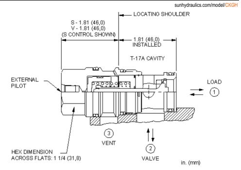
This valve is a pilot to open check valve. It has a non-sealed pilot, a steel seat, and is vented. It allows free flow from the valve (port 2) to the load (port 1) and blocks flow in the opposite direction. Pressure at the external pilot port will open the valve from port 1 to port 2. Pilot pressure needed to open the valve is directly proportional to the load pressure at port 1. The valve is insensitive to pressure at port 2 because the spring chamber references the vent (port 3).
