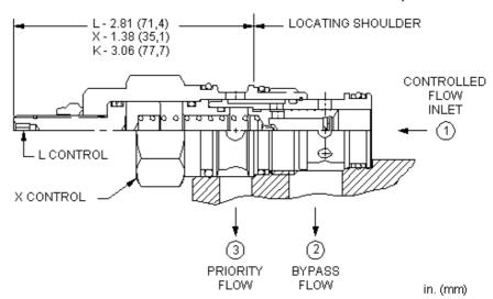
Bypass/restrictive, fixed-orifice, priority flow controls take an input flow at port 1 and use it to satisfy the priority flow at port 3. If the input flow exceeds the priority flow requirement, the excess is bypassed out port 2. The bypass flow may be used in a secondary circuit.
