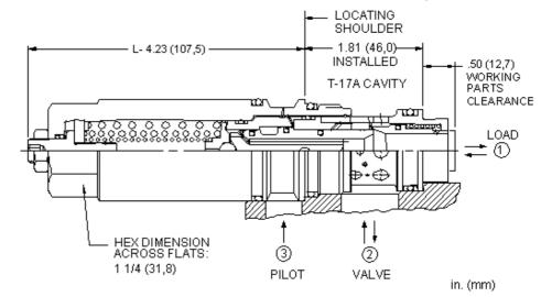
Load reactive, load control valves with pilot assist combine two valves; a check valve and a relief valve. The check valve allows free flow from the directional valve (port 2) to the load (port 1) while a direct-acting, pilot-assisted relief valve controls flow from port 1 to port 2. Pilot assist at port 3 lowers the effective setting of the relief valve at a rate determined by the pilot ratio.
