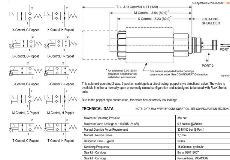
NOTES Please verify cartridge clearance requirements when choosing a Sun manifold. Different valve controls and coils require different clearances.
