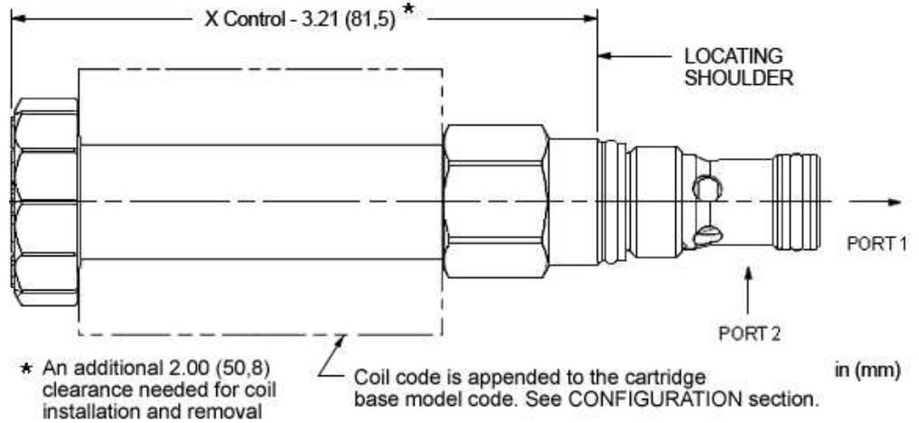
This valve is a pilot-operated, normally closed, electro-proportional throttle with reverse free-flow check. Energizing the coil generates an opening force on the pilot stage which vents the main stage poppet to open proportionally, allowing flow from port 2 to 1. The check will allow flow from 1 to 2 in either the open or closed condition.
