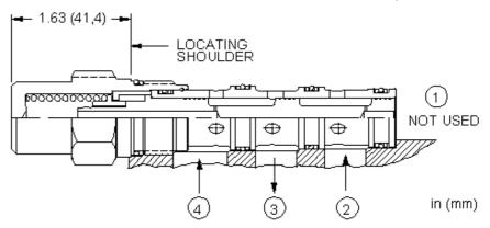
Spring-offset, high-side shuttle cartridges are 2-position valves that have a normal (offset) position that connects the common port (port 3) to work port 4, with work port 2 blocked. When the pressure at port 2 rises above the pressure at port 4, the cartridge shifts to connect the common port to port 2 with port 4 then blocked.
