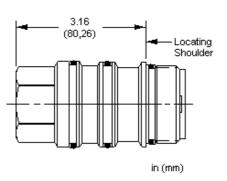
These cavity plugs can be used for both four-port and six-port cavities. When used in four-port cavities (T-21A, T-22A, T-23A and T-24A), ports 1 and 2 remain connected and ports 3 and 4 are blocked. When used in six-port cavities (T-61A, T-62A, T-63A and T-64A), ports 1, 2, 3 and 4 remain connected and ports 5 and 6 are blocked.
