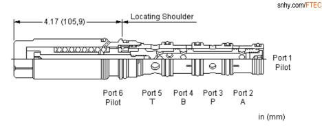
This valve is a 4-way, 3-position proportional directional valve. Work ports 2 and 4 are drained to 5 in the center position and port 3 is closed. Pilot pressure at port 1 opposes the spring and creates a variable metering orifice between ports 3 and 4 that is proportional to the pressure at 1. Piloting 6 opens 3 to 2. The force balance of the flow forces, spring and pilot pressure results in a degree of partial self-compensation as the load pressure changes.
