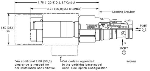
This solenoid controlled, 2-way, 2-position cartridge is a pilot-operated, poppet style directional valve with reverse free flow check. It is available in either a normally open or normally closed configuration. Due to its poppet style construction, it has extremely low leakage.
