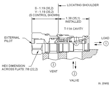
This valve is a pilot to open check valve. It has a non-sealed pilot, a Delrin seat, and is vented. It allows free flow from the valve (port 2) to the load (port 1) and blocks flow in the opposite direction. Pressure at the external pilot port will open the valve from port 1 to port 2. Pilot pressure needed to open the valve is directly proportional to the load pressure at port 1. The valve is insensitive to pressure at port 2 because the spring chamber references the vent (port 3).
