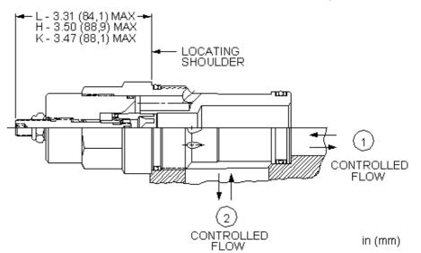
Needle valves are fully adjustable orifices used to regulate flow. They are infinitely adjustable from fully closed up to the maximum orifice diameter. They are not pressure compensated and may be used as flow controls or as shutoff valves.
