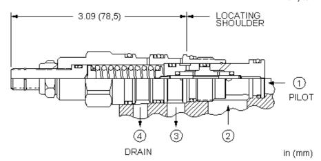
The normally-open, direct-acting 2-way directional cartridge with external drain is a pilot unloading valve used to sense pressure in one circuit to switch or unload a valve in a different circuit. When pressure at port 1 exceeds the setting of the valve, the spool shifts to block port 2 from port 3.
