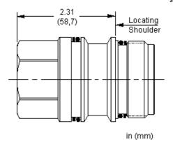
This cavity plug allows ports 1 and 2 to remain open and blocks port 3.
