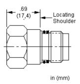
These cavity plugs can be used for both two-port and four-port cavities and allow all ports to remain connected.
