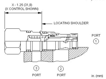
Normally open modulating elements without an internal orifice act as a restrictive compensator to maintain a constant pressure drop across an orifice, regardless of variations in upstream or downstream pressure.
