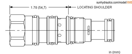
This cavity plug allows flow through ports 1 and 3 and blocks ports 2 and 4.
