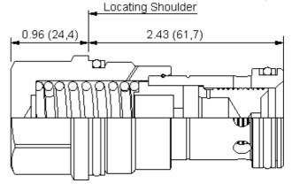
This valve was designed to be used in a parts-in-body, hot oil shuttle assembly. 2 valves, nose to nose, with a pin in between created the low side shuttle.
