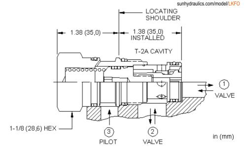
These unbalanced, pilot-to-open logic valves are 2-way switching elements that are spring biased open. Pressure at either work port 1 or 2 will oppose the spring and tend to close the valve while pressure at port 3 will tend to open it. The force generated at port 3, minus the spring force, must be greater than the sum of the forces acting at port 1 and port 2 for the valve to close. NOTE: The pilot area (port 3) is 1.8 times the area at port 1 and 2.25 times the area at port 2.
