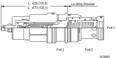
Pilot-operated, anti shock sequence cartridges limit maximum system pressure and also limit the rate of pressure rise. The valve opens and then ramps closed at a constant speed, independent of settings and flows. The adjust screw determines the maximum (relief) setting and the minimum (threshold) setting.
