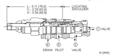
This is a normally closed, balanced poppet, switching element. When pilot pressure is applied to port 3, the poppet remains closed until the pilot pressure reaches the setting established by the integral pilot relief stage, at which point the poppet shifts to the open position.
