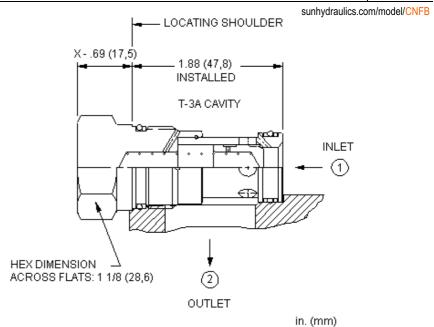
Free-flow, nose-to-side check valves with a bypass orifice allow free flow from port 1 to port 2. A customer specified orifice is included to restrict flow from port 2 to port 1. See technical data below for orifice range.
