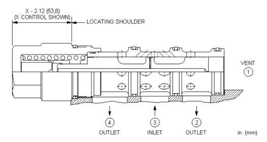
This vent-to-shift diverter valve is a 2-position, 3-way cartridge that is normally open from port 3 to port 4. When port 1 is vented, the pressure differential between port 3 and port 1 exceeds the spring force causing the valve to shift, thereby connecting port 3 to port 2.
