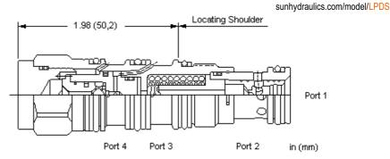
A normally open modulating element, used as a restrictive compensator, ensures a constant pressure drop across an external orifice to create a pressure compensated flow control. The resulting flow remains constant regardless of variations in upstream or downstream pressure.
