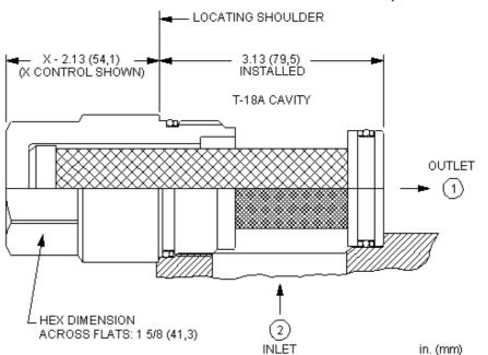
Sun filter elements are available as Surface Type (Last Chance) and Depth Style elements. The flow path is Port 2 to Port 1 and should not be used in reverse, even with a reverse free flow check valve installed. The elements have a high collapse pressure and are intended to be used in line with the system. Filter life will depend on initial system cleanliness and the amount of dirt ingression to the system when operating.
