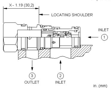
The back-to-back check valve combines two simple check valves into a single cartridge. It connects the work port with the higher pressure to the signal or common port. The signal is sensed at port 3.
