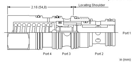
This valve is a 2-way, 2-position proportional throttle. Ports 2 and 3 are normally closed. Pilot pressure at port 1 creates a metering orifice between port 2 and 3 that is proportional to the pressure at 1. The force balance of the flow forces, spring and pilot pressure results in a degree of partial self-compensation as the load pressure changes.
