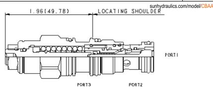
Counterbalance valves with pilot assist are meant to control an overrunning load. The check valve allows free flow from the directional valve (port 2) to the load (port 1) while a direct-acting, pilot-assisted relief valve controls flow from port 1 to port 2. Pilot assist at port 3 lowers the effective setting of the relief valve at a rate determined by the pilot ratio.
