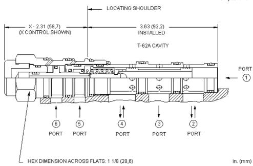
Three-position, 4-way directional cartridges are spring-centered, 6-port directional valves that can be configured from a choice of 10 different spool options. The supply port is port 1 and all ports will accept 5000 psi (350 bar). Capacity for these pilot-to-shift valves is dependent on the spool type specified.
