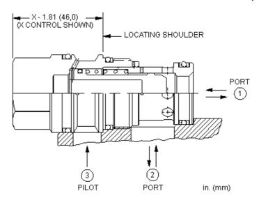
These unbalanced, pilot-to-close logic valves are 2-way switching elements that are spring biased open. Pressure at either work port 1 or 2 will tend to keep the valve open while pressure at port 3 will tend to close it. The force generated at port 3 must be greater than the sum of the forces acting at port 1 and port 2 plus the spring force for the valve to close. NOTE: The pilot area (port 3) is 1.8 times the area at port 1 and 2.25 times the area at port 2.
