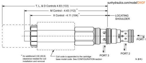
This solenoid-operated 3-way, 2-position cartridge is a direct-acting, poppet-style directional valve. The valve is normally open between port 1 and port 2 with port 3 blocked. Energizing the valve connects port 2 to 3 and blocks port 1. All flow paths are bidirectional and blocked paths are blocked in both directions. Due to the poppet style construction, this valve has extremely low leakage.
