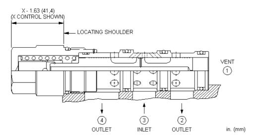
This vent-to-shift diverter valve is a 2-position, 3-way cartridge that is normally open from port 3 to port 4. When port 1 is vented, the pressure differential between port 3 and port 1 exceeds the spring force causing the valve to shift, thereby connecting port 3 to port 2.
