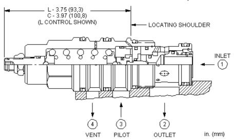
Vented counterbalance valves with pilot assist are meant to control an overrunning load. The check valve allows free flow from the directional valve (port 2) to the load (port 1) while a direct-acting, pilot-assisted relief valve controls flow from port 1 to port 2. Pilot assist at port 3 lowers the effective setting of the relief valve at a rate determined by the pilot ratio. Backpressure at port 2 does not affect the valve setting because the spring chamber references the vent (port 4).
