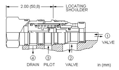
This is a normally closed, balanced poppet, switching element. When the vent port (port 4) is blocked, the poppet remains in the closed position. Venting port 4 shifts it to the open position, provided there is sufficient pressure at port 3.
