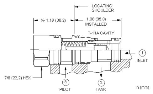
Normally closed modulating elements without an internal orifice act as a bypass compensator to maintain a constant pressure drop across an orifice, regardless of variations in upstream or downstream pressure.
