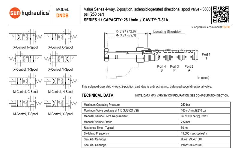
• Please verify cartridge clearance requirements when choosing a Sun manifold. Different valve controls and coils require different clearances. NOTES
