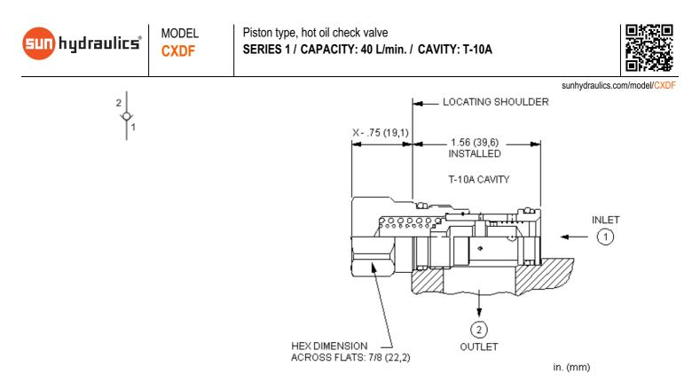
This valve was designed to be used in a parts-in-body, hot oil shuttle assembly. 2 valves, nose to nose, with a pin in between created the low side shuttle.
