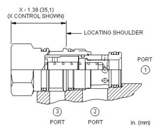
Normally closed modulating elements without an internal orifice act as a bypass compensator to maintain a constant pressure drop across an orifice, regardless of variations in upstream or downstream pressure.
